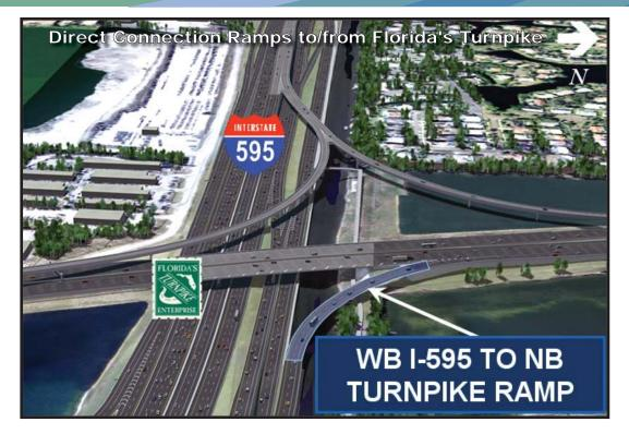
Motorists on the 595Express will have the option of exiting to / entering from the Florida's Turnpike via a direct connection to the Turnpike's median. The direct connection will ease the amount of weaving that currently takes place as I-595 motorists merge on and off of the Turnpike. Along Florida's Turnpike, the southern access point is between Griffin Road and I-595, and the northern location is between I-595 and Peters Road.
